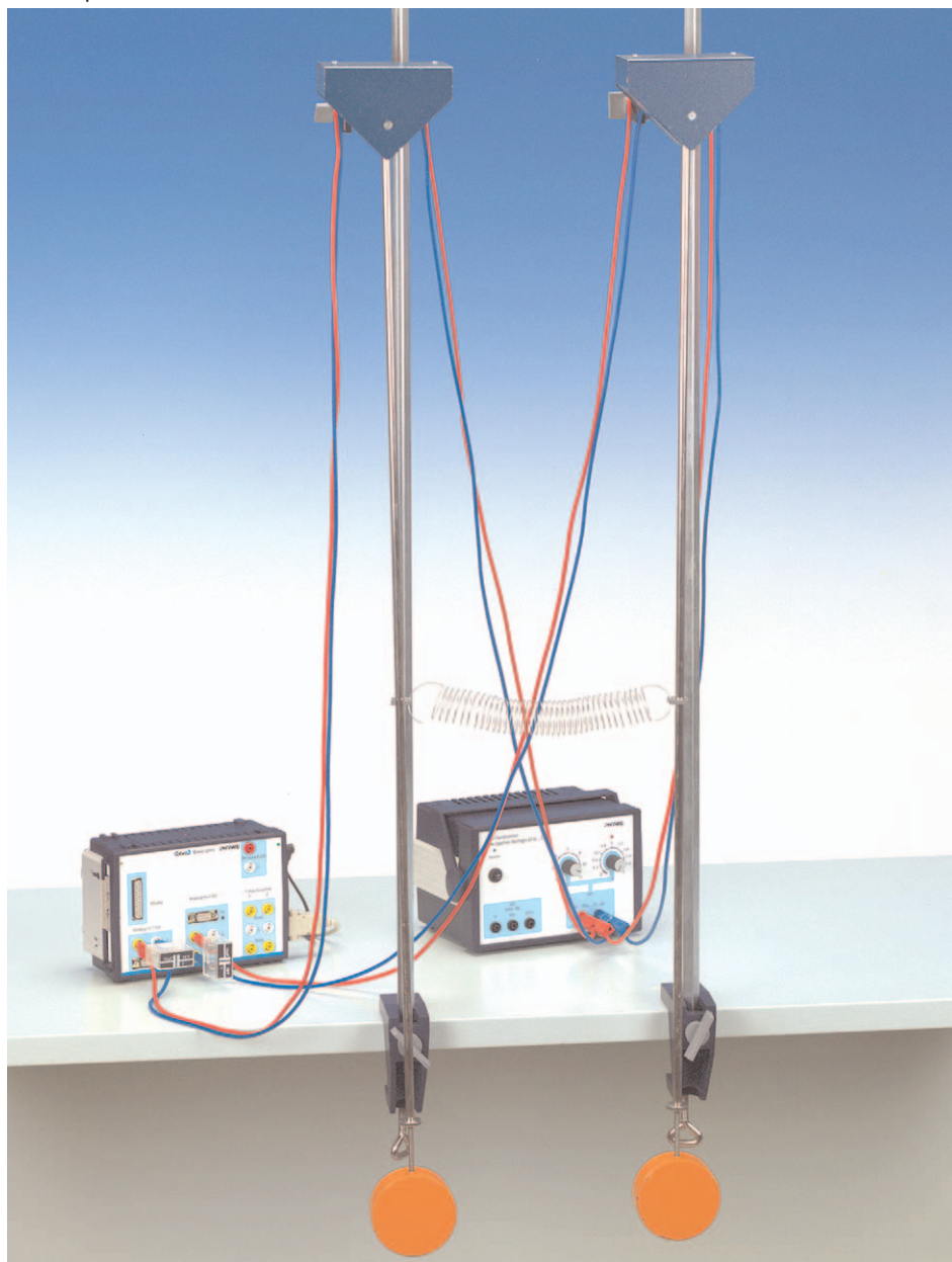
Fig. 1: Experimental set-up for the measurement of the vibrational period of coupled pendula.
